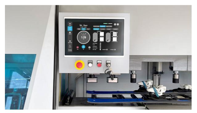
The SF-4 Race service robot is now equipped with a new powerful Beckhoff control. This offers a wide range of new functions and advantages for the machine operator. These include significantly simplified programme and structure creation with an intuitive structure simulator as well as new diagnostic functions and grinding statistics.
